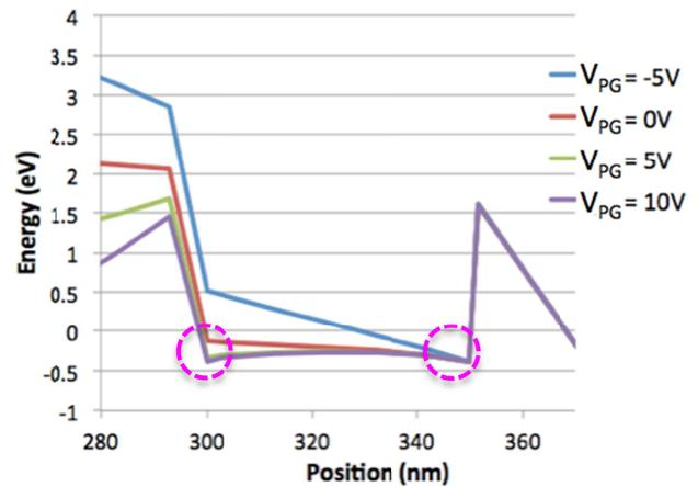
Fig. 4 Simulated conduction band diagrams of dual-gate TFTs in various top gate biases along vertical direction. The bottom gate is biased at a constant voltage of 5V.
