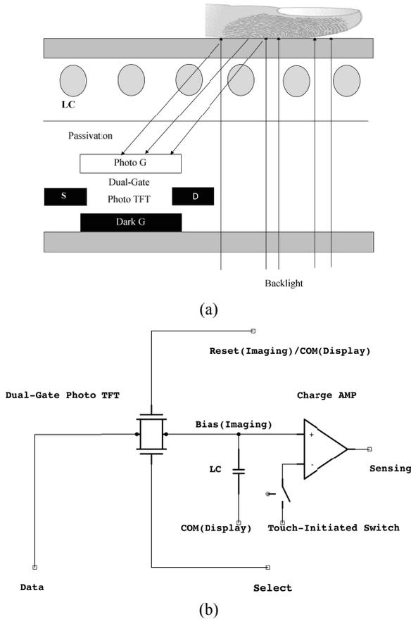
Fig. 2 (a) Schematic diagram of LCD pixel with dual-gate photosensitive TFT as integrated fingerprint sensor; (b) Simplified dual-mode pixel circuit diagram for fingerprint imaging and display driving
