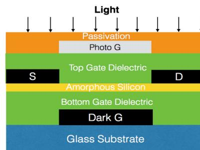
Fig. 1 Cross-sectional structure of an a-Si:H dual-gate photosensitive TFT
