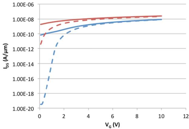
Fig. 5 Simulated transfer characteristics of the bottom TFT at  $V_{PG}=0V$  and  $2V$  with (red) and without (blue) light illumination.
