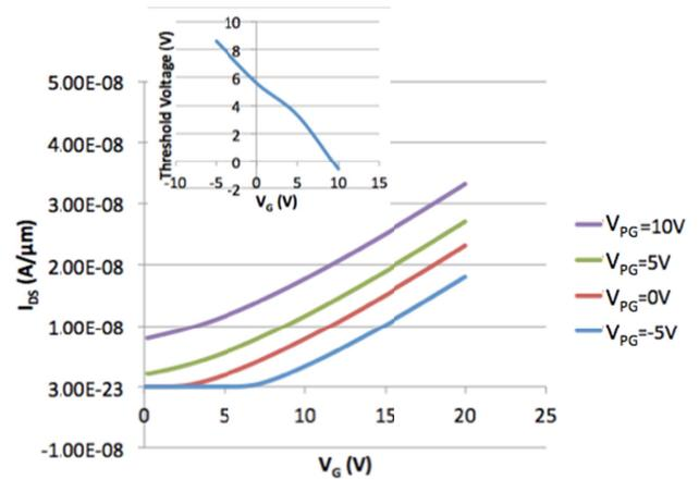
Fig. 3 Simulated IV curves of bottom TFT at different top gate biases.
