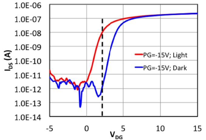
Fig. 6 Transfer characteristics of the fabricated dual-gate photosensitive TFTs with W/L ratio of  $250/20\mu m$ . The process is compatible with BCE TFT process in LCD manufacture. White light source with 3.8 Lux is used for testing.
