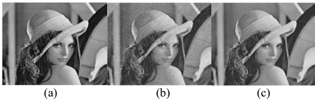
Figure 5. (a) original image, (b) image stored by the traditional SRAM design (SNR = 6.6 dB), and (c) image stored by the proposed MIMS system (SNR = 26.9 dB).
