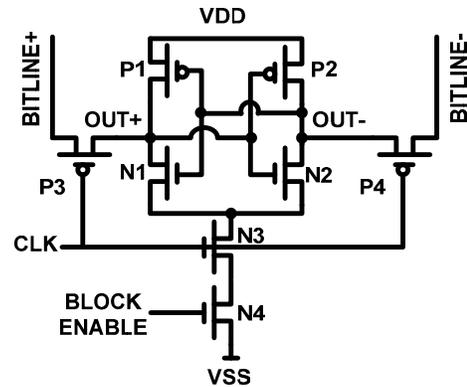
Fig. 1. Latch type sense amplifier (LTSA).
