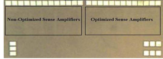
Figure 4. Die photo of the manufactured chip.
