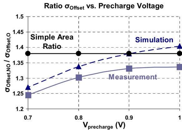
Fig. 6. Comparison of  $\sigma_{\text{Offset}}$  ratio with simple area ratio based on Pelgrom model.
