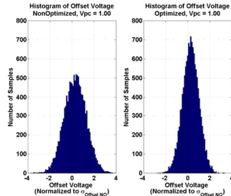
Figure 5. Histogram of input offset voltage (measured).
