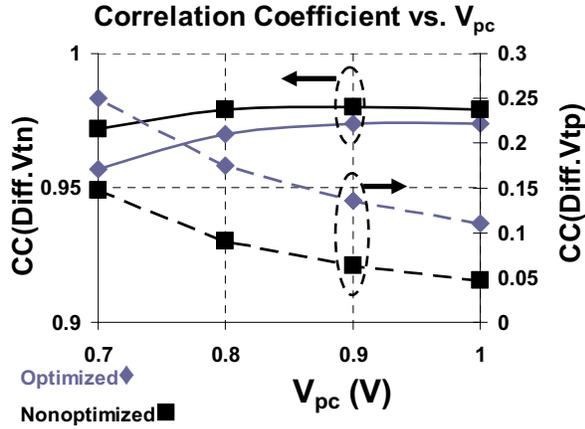
Fig. 3. Correlation Coefficient (CC) of Offset with Diff(V<sub>tn</sub>), Diff(V<sub>tp</sub>).
