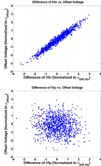
Fig. 2. Offset voltage vs.  $\text{Diff}(V_{tn})$  and  $\text{Diff}(V_{tp})$ ,  $V_{pc}=V_{DD}=1.0V$ .
