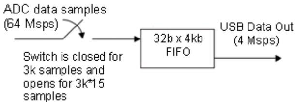
Fig. 2. Schematic of the 64 MSP buffering system
