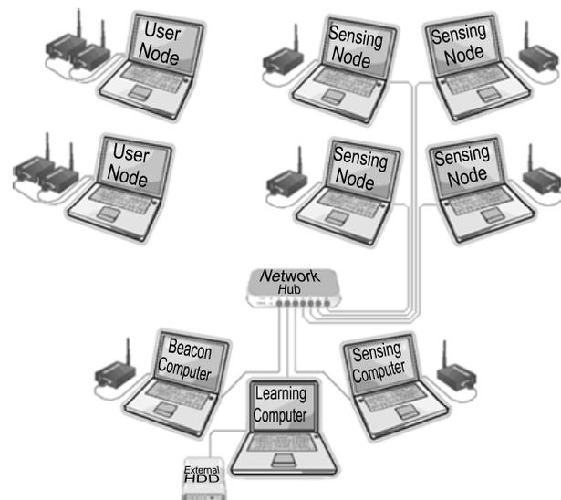
Fig. 1. Diagram of the complete radio network designed by Team Plaid.
