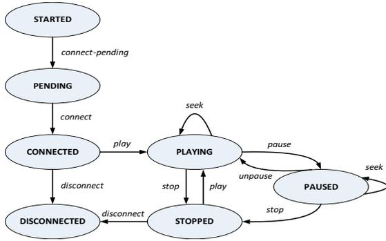
Figure 3: State machine for a connection process
