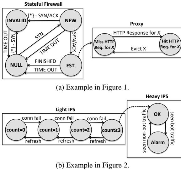
**Figure 5: Modeling DPFs as state machines and service chaining or composition as special conditional transitions between individual state machines.**
