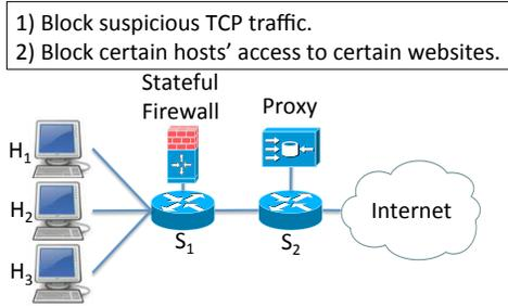
**Figure 1: The stateful firewall maintains a state per TCP connection. The proxy’s state (i.e., cache contents) is determined by the history of observed traffic.**
