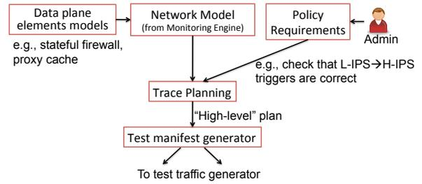
Figure 4: Design of the test traffic planner in FlowTest.
