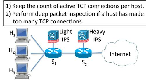
**Figure 2: The test scheme needs to be cognizant of both IPSes states and their event-driven logical connection.**
