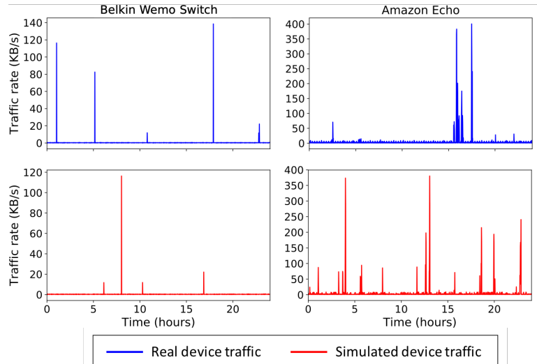
Fig. 7. The start times of spikes in smart home device traffic traces simulated by hidden Markov models could be used to dictate realistic timings of non-activity padding periods in STP.
