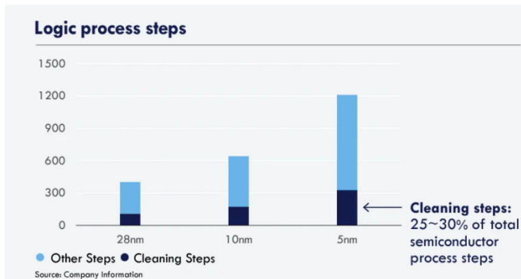
Figure 3: Logic manufacturing process steps comparison between CMOS 28nm, FinFET 10nm, and, FinFET 5nm, technology nodes (from [45]).
