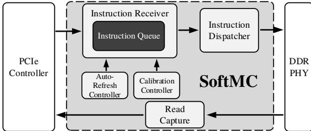
Figure 4: SoftMC hardware architecture.
