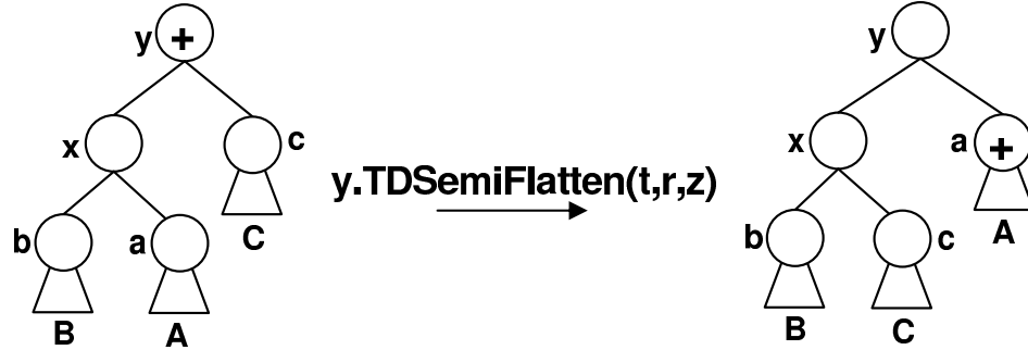
Figure 5.3. Top-down semi-flattening: y , x and a are in the path from t to r . z is y 's parent (not shown). Next invocation is a.TDSemiFlatten(t, r, y) .
