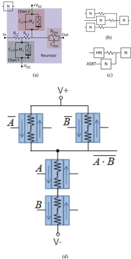
Fig. 3. Neuristor implementation and basic logic gates. (a) Spiking neuristor design based on memristor circuit, (b) AND logic gate, (c) NOT logic gate. The assertion is required to ensure timing of spikes. (d) Oscillatory NAND gate based on magnetic logic gate.
