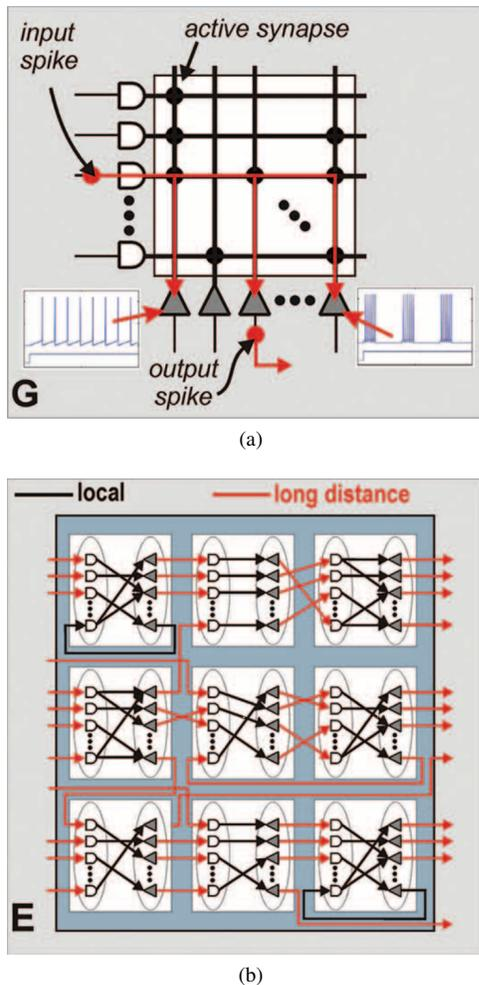
Fig. 2. Functional circuit showing (a) one neuromorphic core and (b) a multiple-core connection of IBM's Synapse chip. The core has 256 fully connected neurons, and the chip consists of an array of 64x64 fully connected cores [8].
