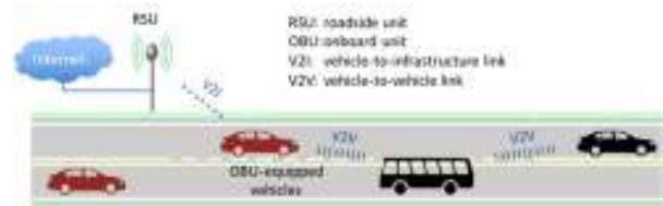
Fig. 1. Vehicular mesh network with roadside infrastructure and multihop connections for Internet access.
