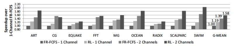
Figure 15: Performance comparison of FR-FCFS and RL-based memory controllers on systems with 6.4GB/s and 12.8GB/s peak DRAM bandwidth
