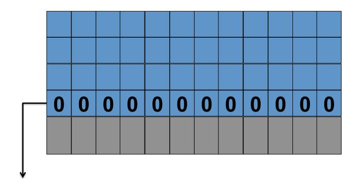
Fix a row at Zero (0.5% loss in capacity)
