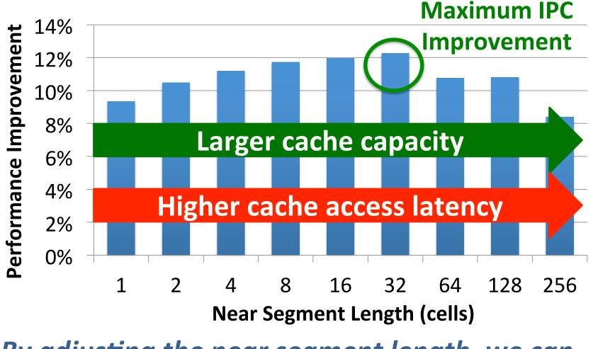
By adjusting the near segment length, we can trade off cache capacity for cache latency
