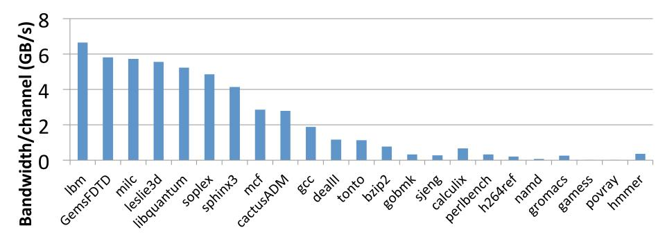
Memory system is provisioned for peak capacity
