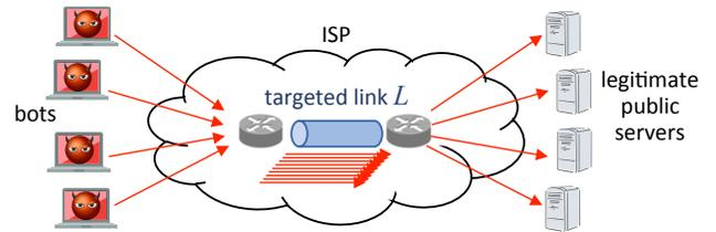
**Fig. 2: An example of link-flooding attacks. Legitimate looking connections between the bots and the legitimate public servers cross the link  $L$  in the ISP [31].**
