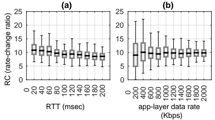
**Fig. 8: Whisker plots representing the rate-change ratios for varying RTT/application-layer data rates when the bandwidth expansion factor  $M = 10$ .**
