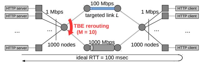
**Fig. 5: Simulation setup.**
