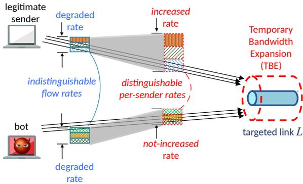
**Fig. 1: Intuition for distinguishing legitimate senders from bots via temporary bandwidth expansion.**
