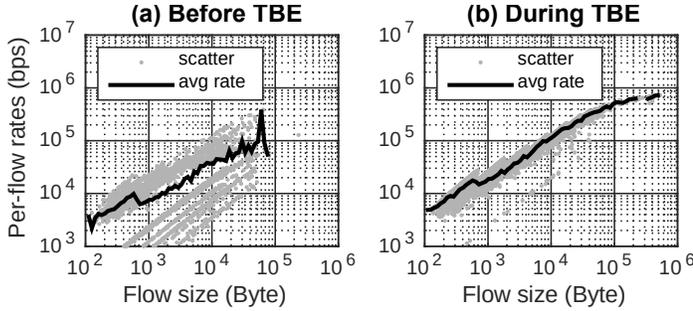
**Fig. 7: Simulated per-flow rates of flows in realistic HTTP web traffic (a) before and (b) during TBE with bandwidth expansion factor  $M = 10$ .**
