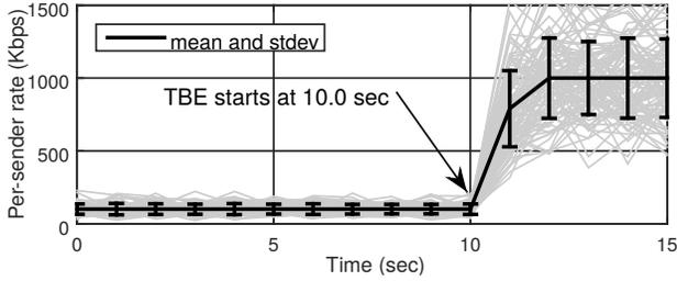
**Fig. 6: An example per-sender rate change measurements of randomly selected 100 legitimate senders with mean and standard deviation when the bandwidth expansion factor  $M = 10$ .**
