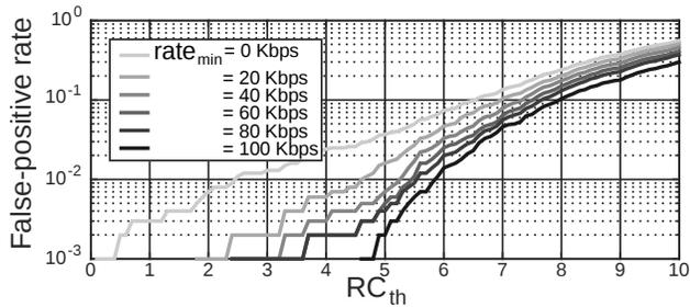
**Fig. 9: False-positive rate for varying rate-change ratio thresholds ( $RC_{th}$ ) and minimum per-sender rates ( $rate_{min}$ ).**
