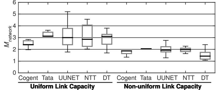
**Fig. 14:  $M_{network}$  values for the five ISPs in two link-bandwidth models.**
