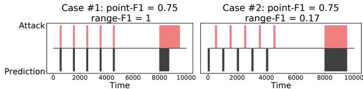
**Fig. 4.** Two detection examples: in each case, the x-axis represents time and the y-axis shows attacks (top, red) and attack predictions (bottom, grey). In the example on the left (case 1), all attacks are detected with no false positives, while in the example on the right (case 2) only one attack is detected, with five false positives; yet, the point-F1 scores are the same.
