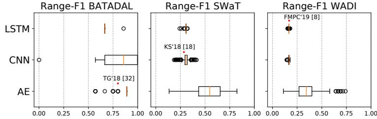
**Fig. 5.** The final range-F1 scores of each model when trained and tuned on 3 experimental ICS datasets. For each dataset, a selected model hyperparameter setting from prior work is included for comparison.
