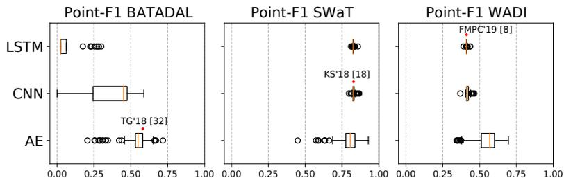
**Fig. 3.** The final point-F1 scores of each model when trained and tuned on three experimental ICS datasets. For each dataset, a model hyperparameter setting from prior work is included for comparison. When using the point-F1, the performance of AEs vary greatly, and most LSTM and CNN configurations perform similarly.
