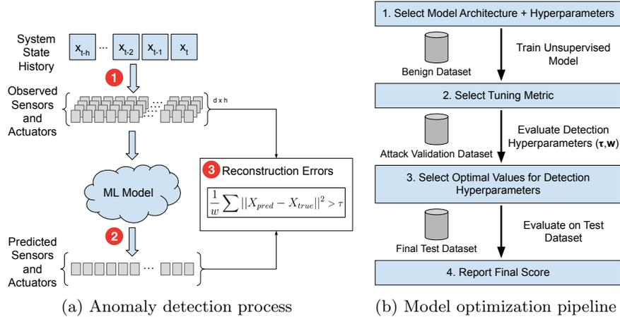
**Fig. 2.** The anomaly-detection process is shown on the left: a sequence of system states is reconstructed by an ML model, and high reconstruction errors are used to identify anomalies. The optimization pipeline for the anomaly-detection process is shown on the right, with each optimization step and its relevant datasets.
