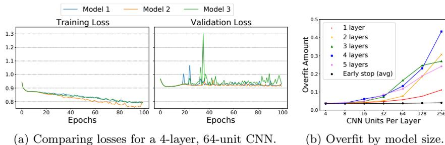
**Fig. 6.** On left (a): the training and validation loss for a 4-layer, 64-unit CNN, across random seeds. On right (b): the average overfit amount without early stopping, shown for all CNN sizes, compared to the average overfit amount for all layers with early stopping.
