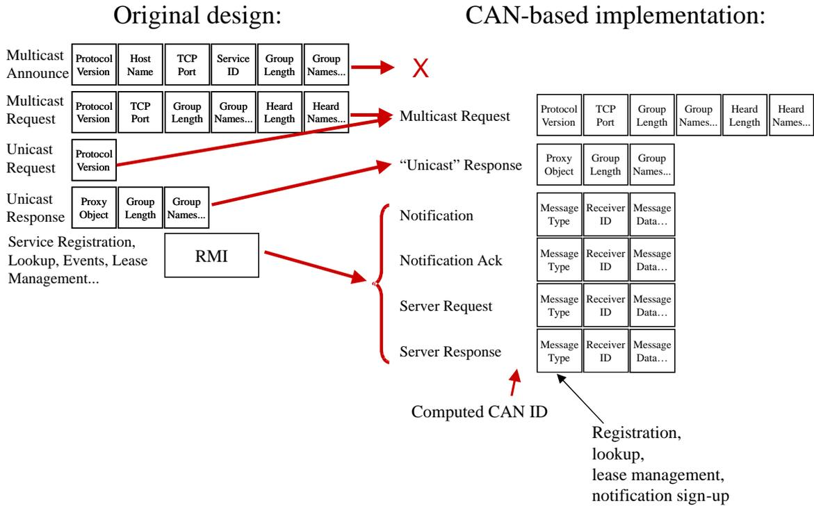
Figure 8: Original Jini modified to work on CAN
