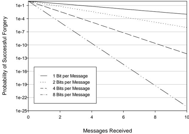
**Figure 2. Probability of successful forgery for one, two, and eight bit MACs over ten messages.**
