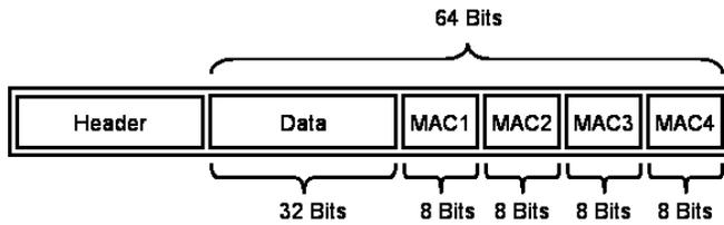
**Figure 1. Example packet containing 32 bits of message data and four 8-bit MACs, for four receivers.**
