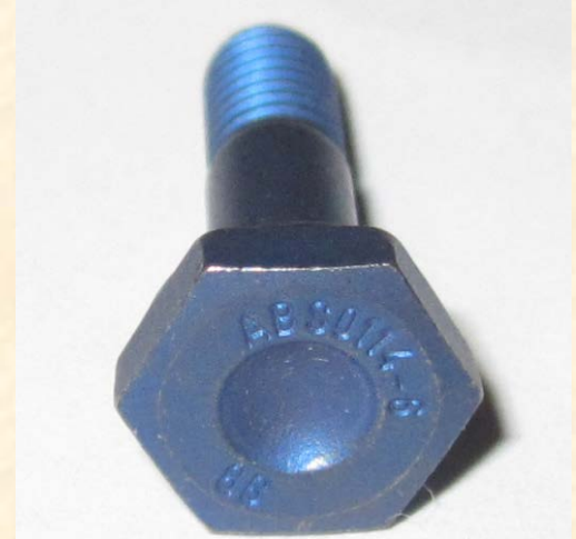
Airbus A-380 bolt with part tracking information. (Size: 2 cm x 1 cm)
