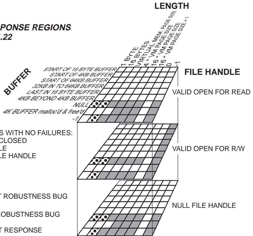
Figure 3. Response regions for *write()* system call on QNX 4.22. Both Restart and Silent robustness gaps occur in three different File Handle cases.
