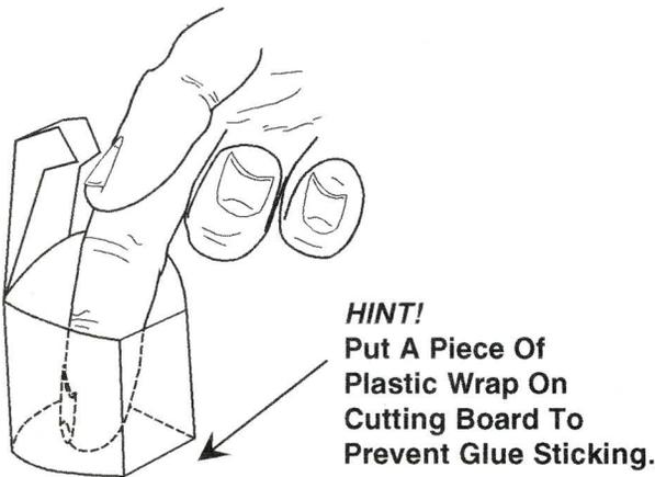
**22.** Check To Make Sure All Tabs Are Glued Flat To The Front Of Cowl. Reglue If Needed. Then, Trim The Bottom Tab Flush With Side.
