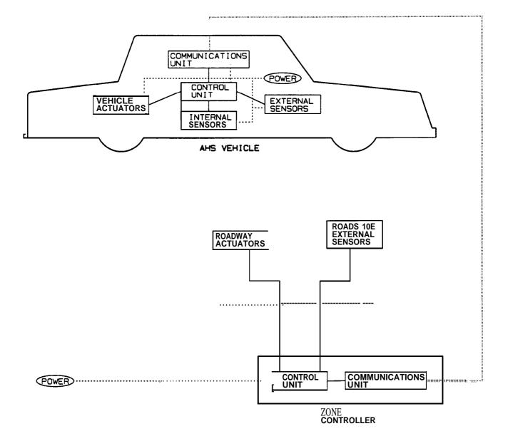
Figure8. AI- R3systemarchitectu reschematic.
