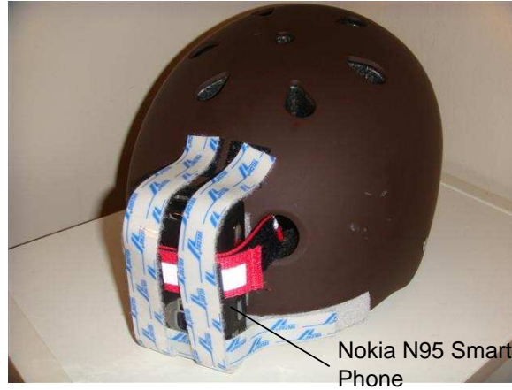
Fig. 1. Sensor helmet for collecting activity data.
