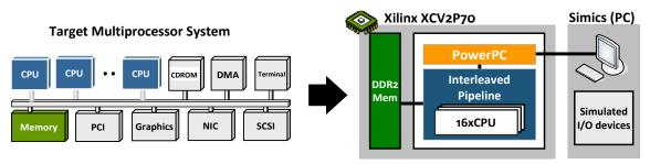
Figure 5 Allocating components for hybrid simulation in the BlueSPARC simulator
