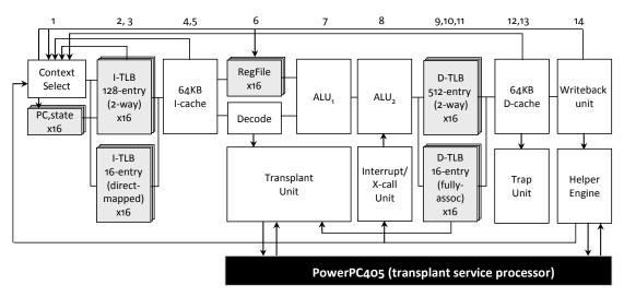
Figure 7 The BlueSPARC engine: a 14-stage instruction-interleaved pipeline
