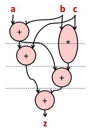
delay=4 using 1 adder and 1 multiplier
