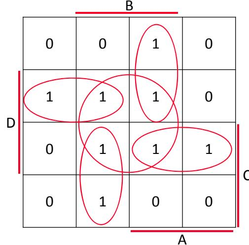
Following the simple K-map recipe will result in a redundant cover in this example.
