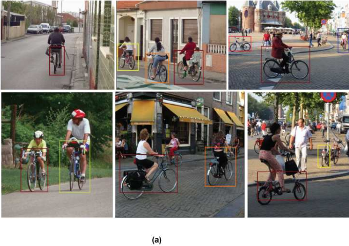
Fig. 5. Examples of detection with our three-component bicycle model (a), PR curves for three detectors (b). The red plot shows the response for the three-component model trained with PASCAL2009 and our dataset and the blue plot and green plot show the response for two-component model and one-component model, respectively, trained with the same dataset.
