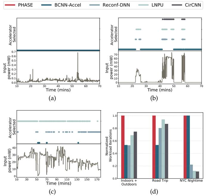
Fig. 3: Timeline of our simulation on three different input traces: (a)Indoors+Outdoors, (b) Road trip and (c) NYC night-time. (d) shows the total iterations of AlexNet inference completed by the different systems, normalized to the PHASE-serial architecture.
