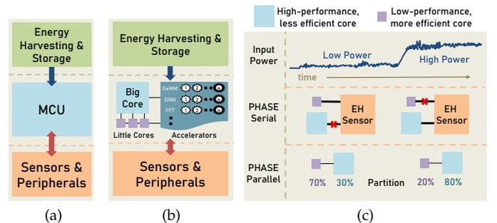
Fig. 1: (a) shows a typical energy-harvesting architecture, with a simple processing core. (b) shows our PHASE architecture with heterogeneous single-workload accelerators and cores. (c) shows how PHASE-serial and PHASE-parallel architectures select fastest architectural configuration depending on input power.
