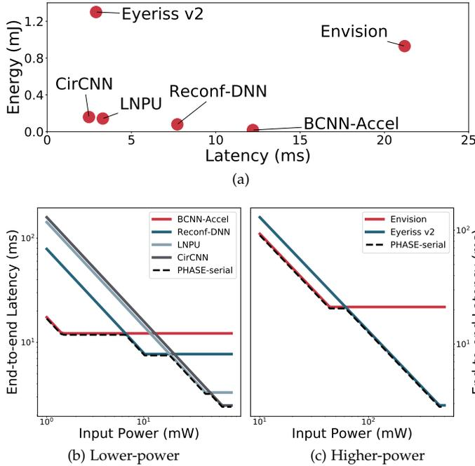
Fig. 2: (a) Energy vs Latency for different DNN accelerators. (b) and (c) End-to-end inference latency vs input power for different accelerators.
