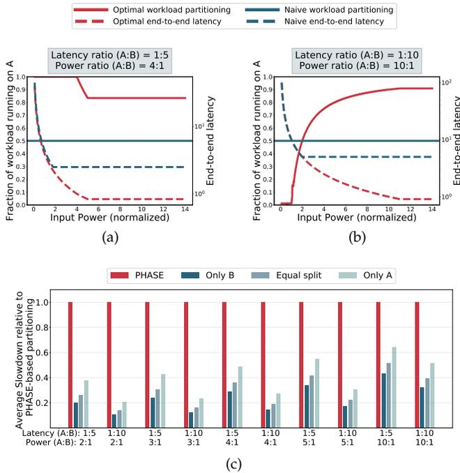
Fig. 4: (a) and (b) compare the end-to-end workload latencies of two PHASE-parallel architectures with a fixed naive 50 : 50 partitioning, for different input power levels. (c) shows the average slowdown of different naive partitionings compared to our PHASE-based partitioning for different PHASE-parallel architectures.
