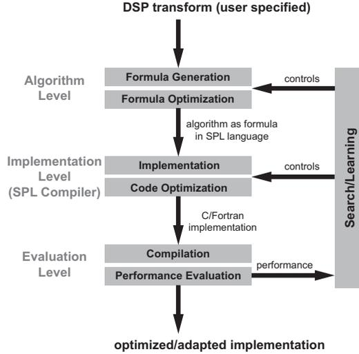
Figure 4. The program generator Spiral.
