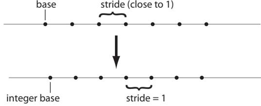
Figure 3. The projection of the real-valued indices of the Cartesian grid onto the integer-valued indices of the Polar Annulus requires resampling. We compute base and stride values for each cross-range and range line based on the projection geometry.
