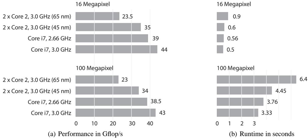
Figure 5. Performance and corresponding runtime of computer-generated SAR implementations on various Intel quadcore systems with large pages. The results on Core i7, 3.0 GHz are “virtual,” i.e., obtained by linearly scaling the measured results on Core i7, 2.66 GHz.
