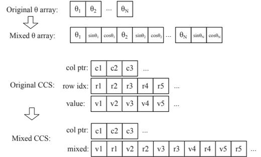
Figure 12: Optimizing data structure (upper: new  $\theta$  array, lower: new CCS)
