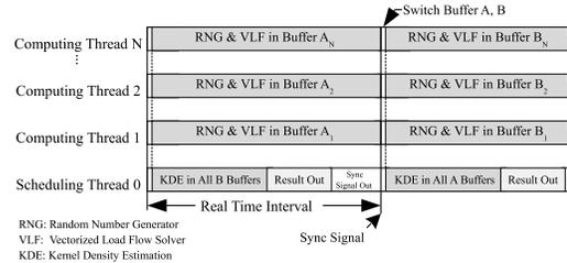
Figure 7: Real time multi-thread MCS on multicore
