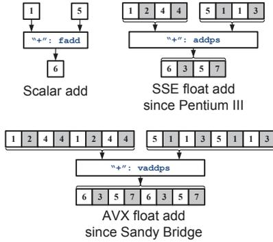
**Figure 3: Illustration of SIMD operation**
