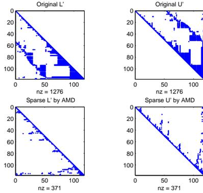
Figure 10: LU of IEEE118's  $\mathbf{B}'$ : LU used in Matpower (top) and sparse LU using AMD (bottom)
