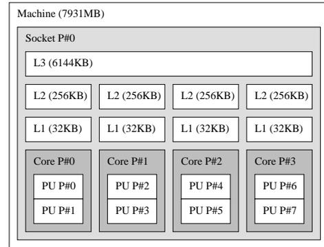
**Figure 1: Core i7 2670QM: 4 physical cores, 3 levels cache (L1–L3), 8 GB memory**
