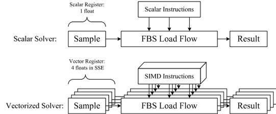
Figure 6: Vectorization of load flow solver for MCS
