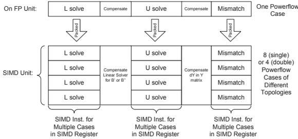
Figure 15: Scalar (upper) and SIMD (lower) model.
