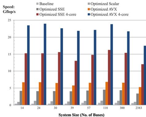
**Figure 14: Optimization impact on computational speed (on Core i7 2670QM)**
