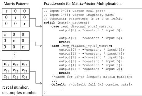
Figure 5: Pattern-based optimized sparse matrix-vector multiplication.
