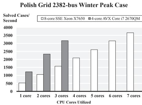
**Figure 18: Thread pool performance of Polish 2383-bus system on different machines**
