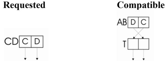
**Figure 4: Compatible Fusion.** The vectorization process requests a fusion  $CD = (C,D)$ . The existing fusion  $AB = (D,C)$  is used as input operand to a swap instruction whose output  $T$  can be used whenever  $CD$  is needed.
