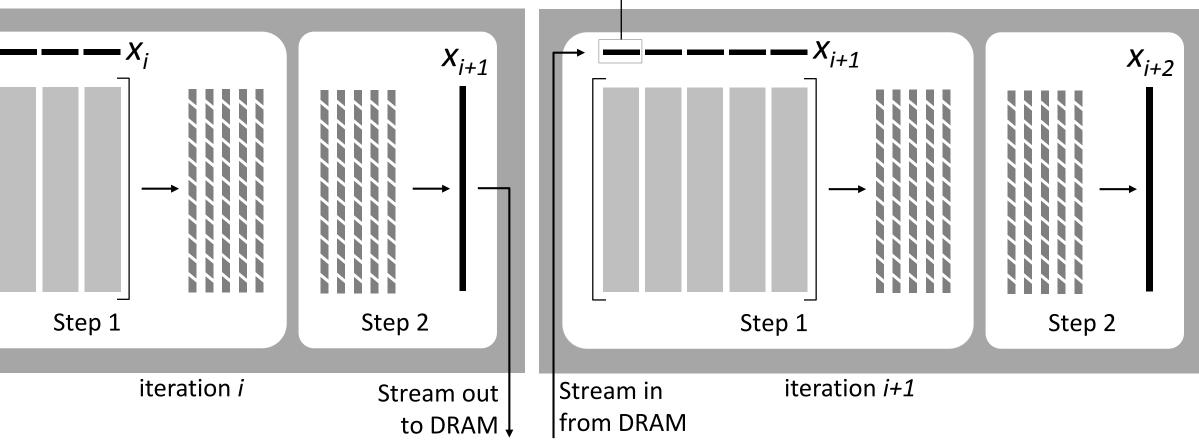
Two-Step SpMV is conducted independently in each iteration of PageRank **Q** Resultant vector of one iteration is the source vector of the next, communicated via DRAM **□** Either Step1 or Step2 is conducted at any given time, keeping other part of the circuit inactive
