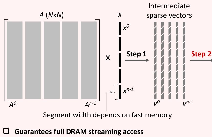
Reduces off-chip traffic and Enables high bandwidth utilization **Requires custom hardware for efficient multi-way merge**
