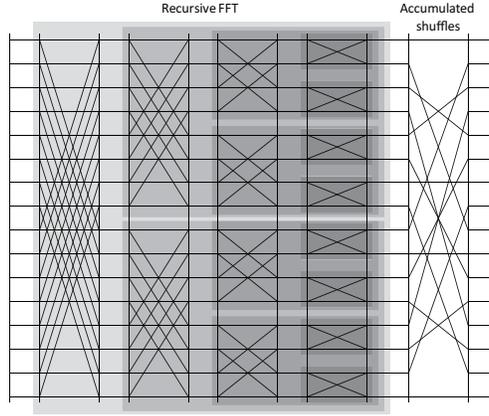
$$(\text{DFT}_2 \otimes I_8) T_8^{16} \left( I_2 \otimes \left( (\text{DFT}_2 \otimes I_4) T_4^8 \left( I_2 \otimes \left( (\text{DFT}_2 \otimes I_2) T_2^4 \left( I_2 \otimes \text{DFT}_2 \right) L_2^4 \right) \right) L_2^8 \right) \right) L_2^{16}$$
