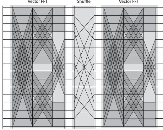
$$\left( ((\text{DFT}_2 \otimes I_2) T_2^4 (I_2 \otimes \text{DFT}_2) L_2^4) \otimes I_4 \right) L_4^{16} T_4^{16} \left( ((\text{DFT}_2 \otimes I_2) T_2^4 (I_2 \otimes \text{DFT}_2) L_2^4) \otimes I_4 \right)$$
