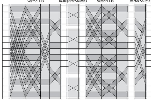
$$\left( ((\text{DFT}_2 \otimes I_2) T_2^4 (I_2 \otimes \text{DFT}_2) L_2^4) \otimes I_2 \right) \otimes I_2 \Big) T_4^{16} \left( I_2 \otimes (L_2^4 \otimes I_2) (I_2 \otimes L_2^4) ((\text{DFT}_2 \otimes I_2) T_2^4 (I_2 \otimes \text{DFT}_2) L_2^4) \otimes I_2 \right) (L_2^8 \otimes I_2)$$
