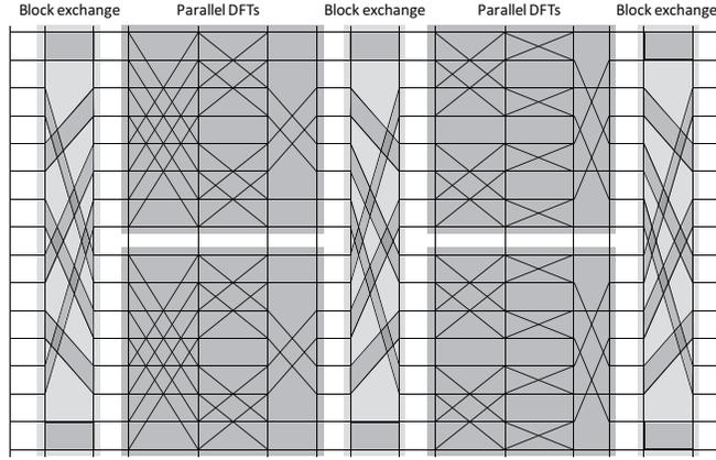
$$(L_4^8 \otimes I_2) \left( I_2 \otimes \left( (\text{DFT}_2 \otimes I_2) T_2^4 (I_2 \otimes \text{DFT}_2) L_2^4 \right) \otimes I_2 \right) (L_2^8 \otimes I_2) T_4^{16} \left( I_2 \otimes \left( (\text{DFT}_2 \otimes I_2) T_2^4 (I_2 \otimes \text{DFT}_2) \right) R_2^8 \right) (L_2^8 \otimes I_2)$$
