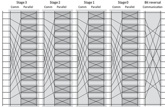
$$\left( L_2^{16} (I_8 \otimes \text{DFT}_2) D_0^{16} \right) \left( L_2^{16} (I_8 \otimes \text{DFT}_2) D_1^{16} \right) \left( L_2^{16} (I_8 \otimes \text{DFT}_2) D_2^{16} \right) \left( L_2^{16} (I_8 \otimes \text{DFT}_2) D_3^{16} \right) R_2^{16}$$
