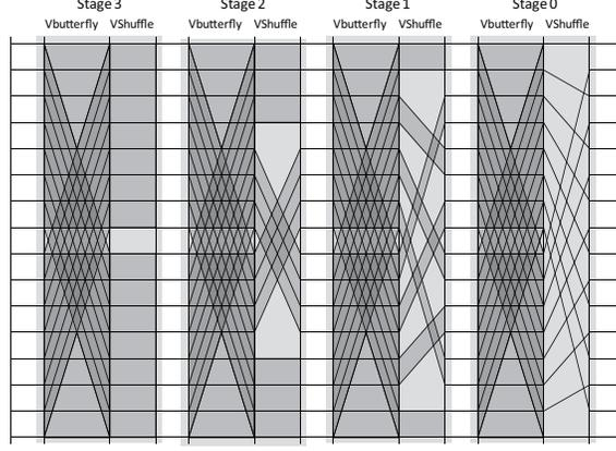
$$\left( (\text{DFT}_2 \otimes I_8) D_0^{16} (L_2^2 \otimes I_8) \right) \left( (\text{DFT}_2 \otimes I_8) D_1^{16} (L_2^4 \otimes I_4) \right) \left( (\text{DFT}_2 \otimes I_8) D_2^{16} (L_2^8 \otimes I_2) \right) \left( (\text{DFT}_2 \otimes I_8) D_3^{16} (L_2^{16} \otimes I_1) \right)$$
