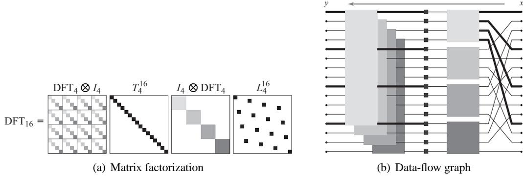
**Figure 2:** Cooley-Tukey FFT (8) for  $16 = 4 \times 4$  as matrix factorization and as (complex) data-flow graph (from right to left). Some lines are bold to emphasize the strided access (figure from [5]).
