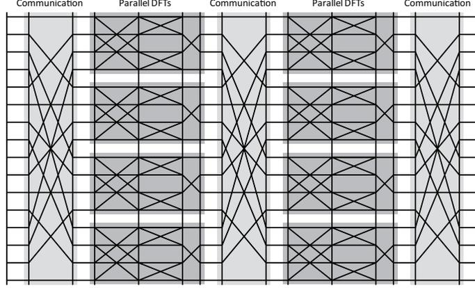
$$L_4^{16} \left( I_4 \otimes \left( (\text{DFT}_2 \otimes I_2) T_2^4 (I_2 \otimes \text{DFT}_2) L_2^4 \right) \right) L_4^{16} T_4^{16} \left( I_4 \otimes \left( (\text{DFT}_2 \otimes I_2) T_2^4 (I_2 \otimes \text{DFT}_2) L_2^4 \right) \right) L_4^{16}$$
