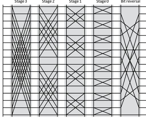
$$\left( (I_1 \otimes \text{DFT}_2 \otimes I_8) D_0^{16} \right) \left( (I_2 \otimes \text{DFT}_2 \otimes I_4) D_1^{16} \right) \left( (I_4 \otimes \text{DFT}_2 \otimes I_2) D_2^{16} \right) \left( (I_8 \otimes \text{DFT}_2 \otimes I_1) D_3^{16} \right) R_2^{16}$$
