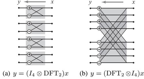
**Figure 1:** Dataflow (right to left) of a block parallel and its “dual” vector parallel construct (figure from [5]).
