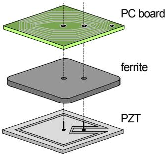
Figure 3. Design of the inductively coupled transducer.
