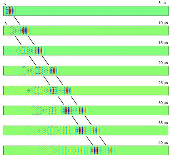
Figure 3. Simulations showing evolution of a pulse train excited with a center frequency of 1000 kHz. The leading nearly-longitudinal pulse decays in amplitude while trailing pulses gain in amplitude. The color indicates the  $x$  displacement.
