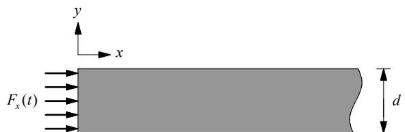
Figure 1. Plate of thickness  $d$  excited by a time-dependent force  $F_x(t)$  normal to the edge.
