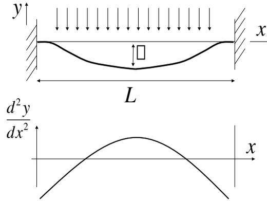
**Figure 7.** Drawing of beam deflection and strain.
