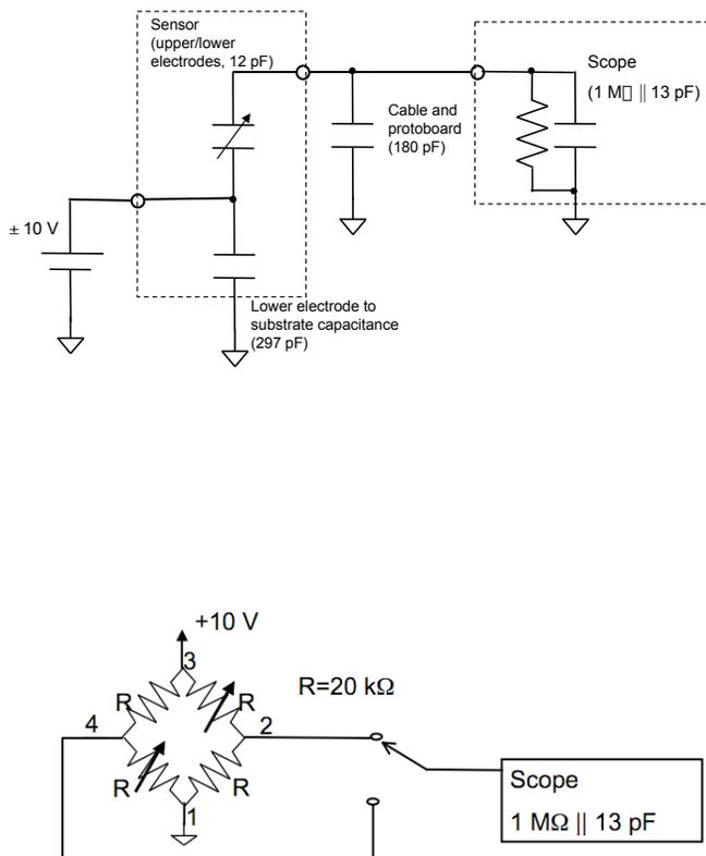
**Figure 4.** Measurement connections for capacitive and piezoresistive sensors.
