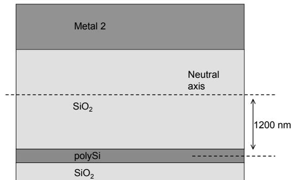
**Figure 2.** Cross section of beam showing thickness of metal and oxide layers, and location of polysilicon (which forms the piezoresistors).
