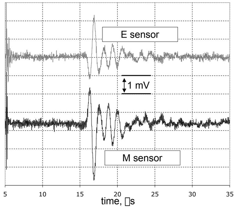
**Figure 5.** Waveforms (8x averaging) measured from piezoresistive and capacitive sensors, with source 16 mm from surface of sensor.
