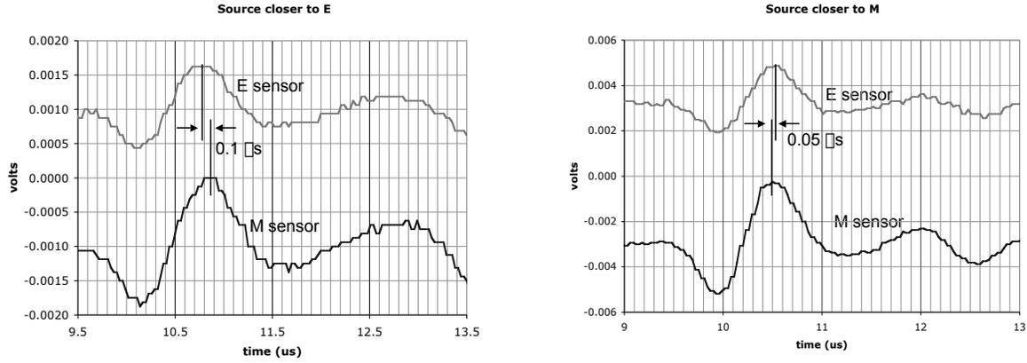
**Figure 6.** Pulse (256x averaging) arriving at slightly different times for the two sensor elements, for two different source positions.
