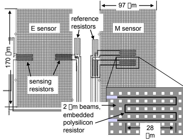
**Figure 3.** Layout of type **E** (left) and type **M** piezoresistive bridges on diaphragms. Crosshatch design is the diaphragm, and surrounding white area is solid (location of reference resistors).
