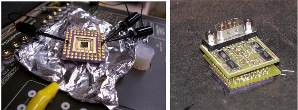
Figure 5. (a) 2006 MEMS device mounted in pin grid array package; (b) 2006 MEMS sensor system, with electronics, on steel plate.
