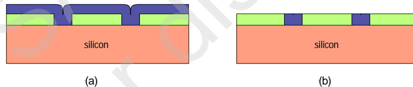
Figure 2.6. Chemical mechanical polishing: (a) before polishing and (b) after polishing.
