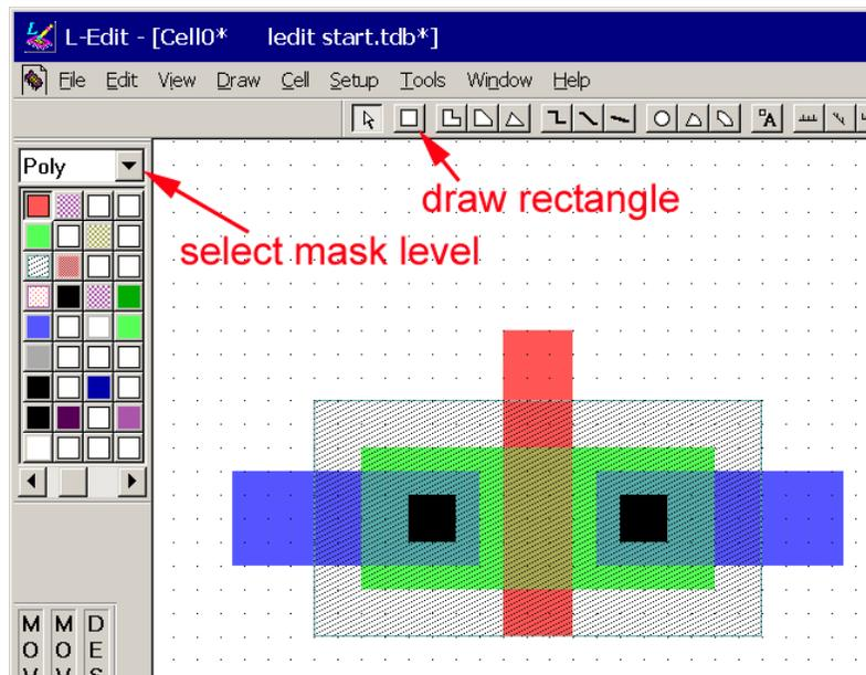
Figure 3. Detail showing menu for selection of mask level to be drawn and button to select the *draw rectangle* option. Note the arrow just to the left of the *draw rectangle* button for selecting polygons.
