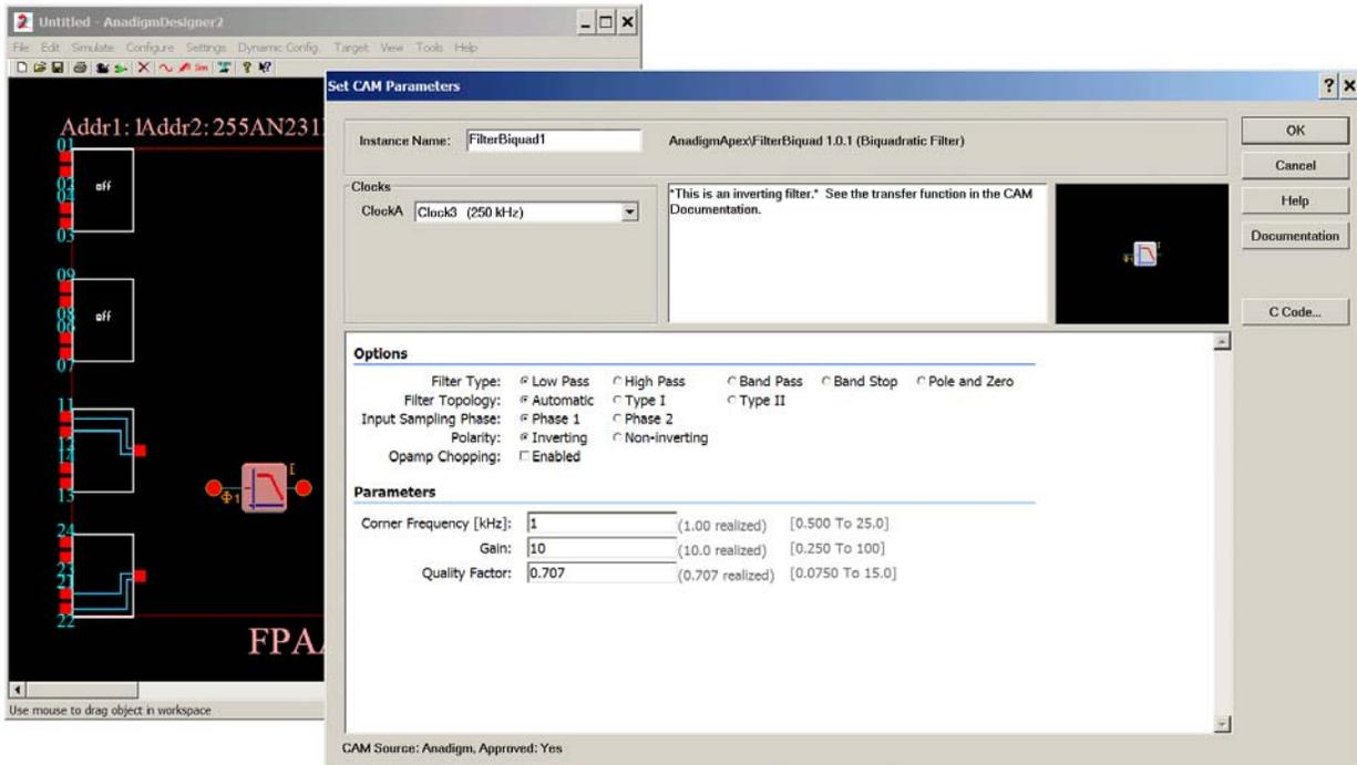
Fig. 4. Configuration screen for biquadratic filter CAM.
