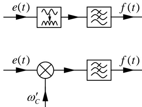
Figure 5. Block diagrams for detection of AM (top) and DSB, USB, and LSB signals (bottom). The first block in the AM detector is a rectifier.
