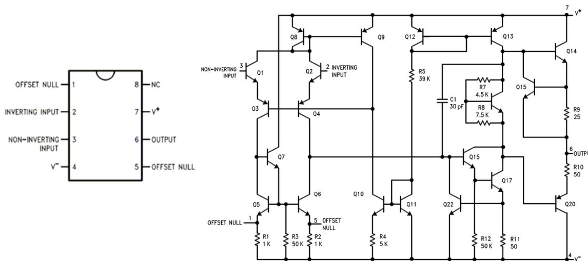
Figure 1. Op amp pinout and internal circuit diagram.
