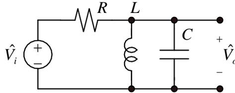
Figure 4. A filter circuit.
