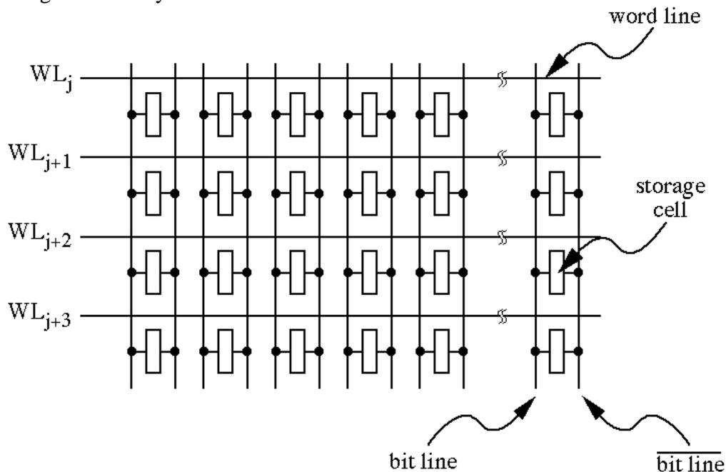
Figure 1. Schematic layout of an SRAM.
