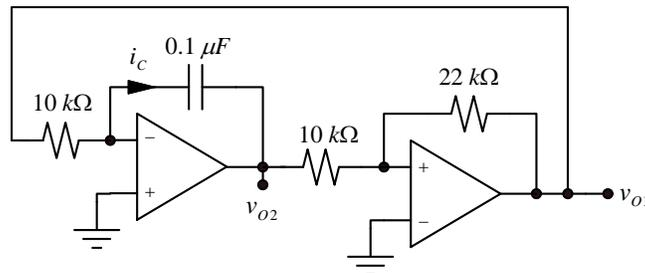
Figure 4. Ramp generator circuit.
