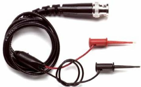
**Exercise #4.** With the probe properly compensated determine the rise time (defined as the time required to get from 10% of the final value to 90% of the final value) of the built-in square wave. **Enter the result in your notebook.**
