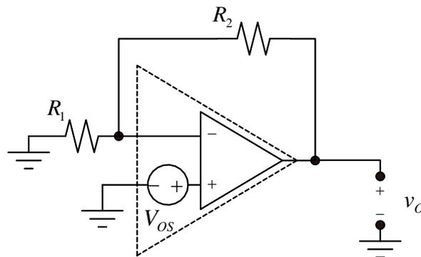
Fig. 5. Real op amp with an additional voltage source to model the offset voltage.
