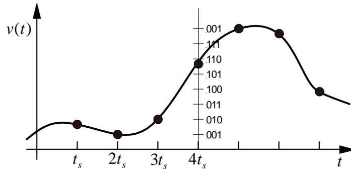
Figure 2. Analog to digital conversion of a signal.
