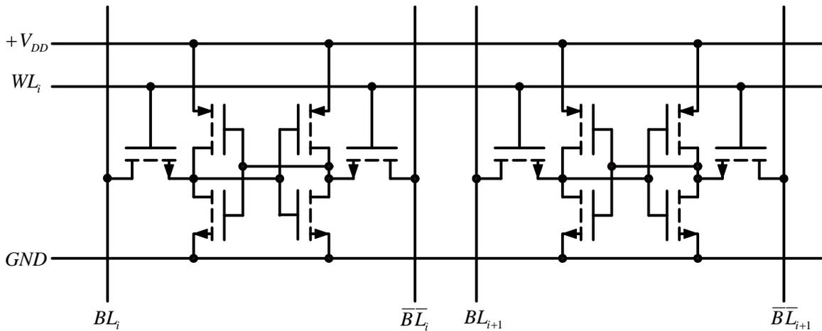
Figure 2. Detailed circuit diagram of two SRAM storage cells.
