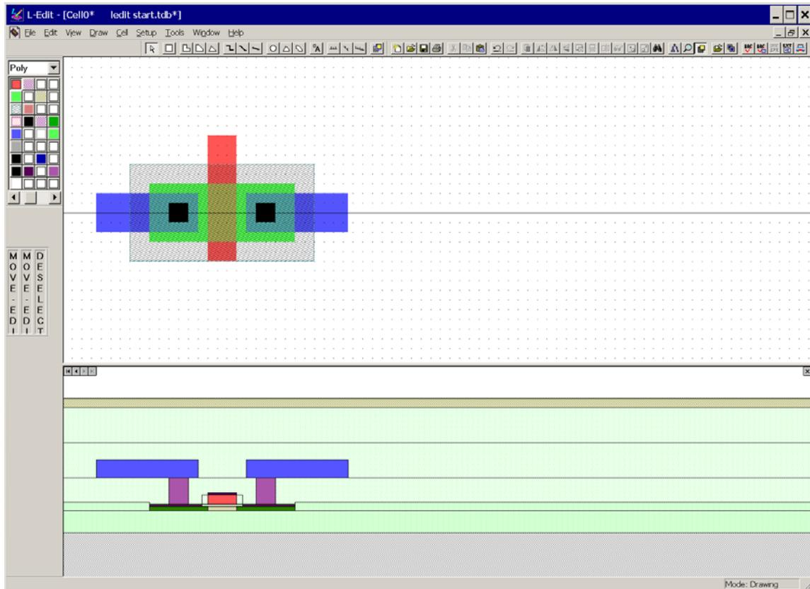
Figure 8. A cross section drawn by L-edit along the line selected.
