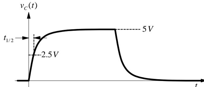
Fig. 2. Waveform resulting from step excitation of RC circuit.
