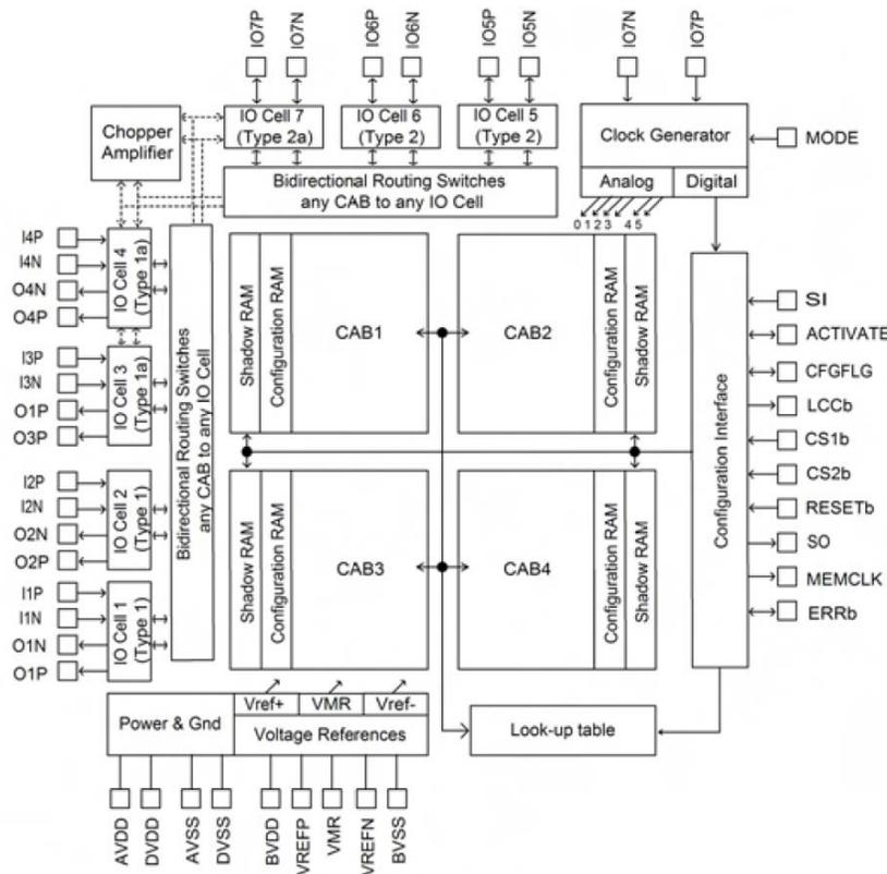
Figure 1. Block diagram of the analog signal processor chip.
