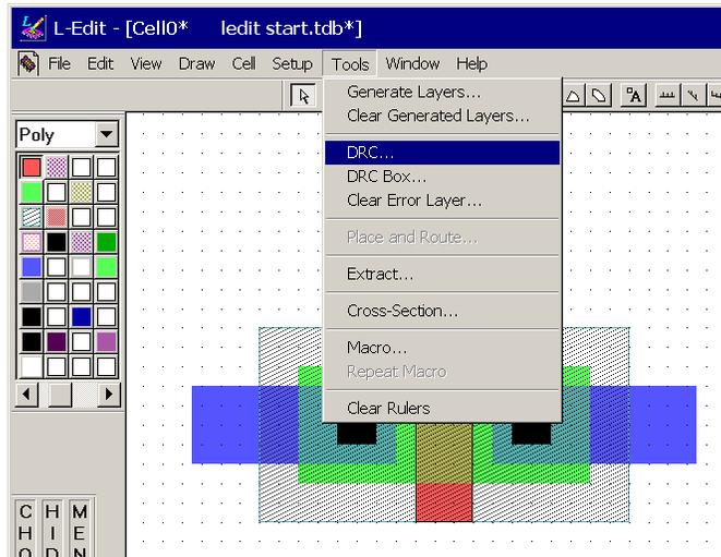
Figure 4. Initiating the DRC check.
