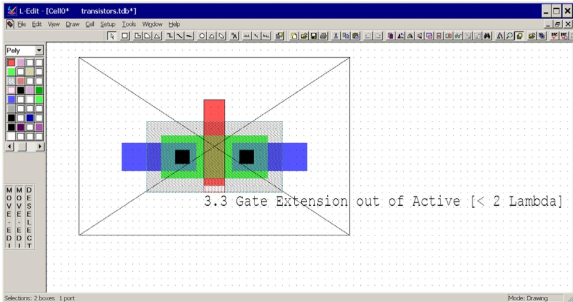
Figure 6. After selecting the error location the description of the error appears.
