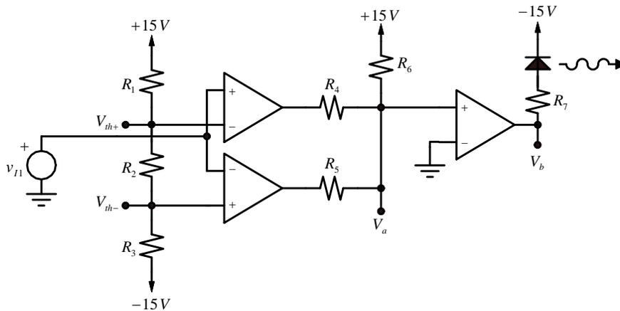
Figure 1. Peak detector circuit.
