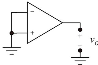
Fig. 4. Op amp with zero differential voltage input.
