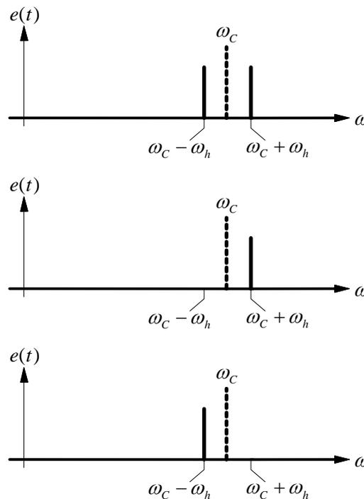
Figure 4. Spectra from modulation with a single frequency sinusoid: (top) double-sideband suppressed carrier; (middle) upper sideband and (bottom) lower sideband. The dashed line indicates the the carrier frequency, which is not present in the modulated output.
