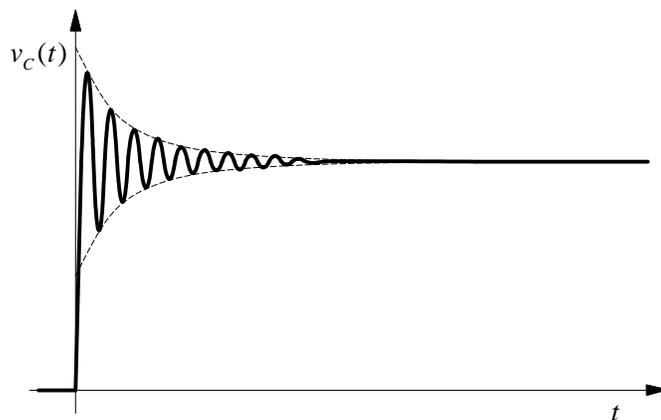
Fig. 6. Step response of  $RLC$  circuit (underdamped).
