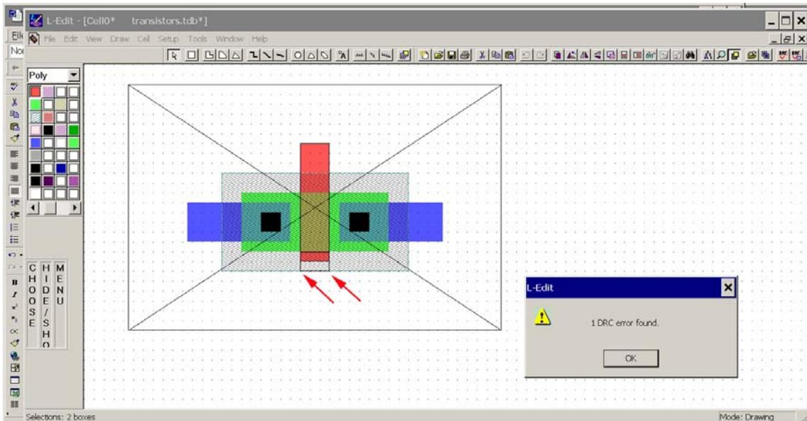
Figure 5. Result of a DRC check (one error present). Arrows show the solid lines indicating the error location.
