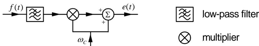
Figure 1. Block diagram showing system for amplitude modulation. The low-pass filter is not necessary if the input signal is already band-limited.
