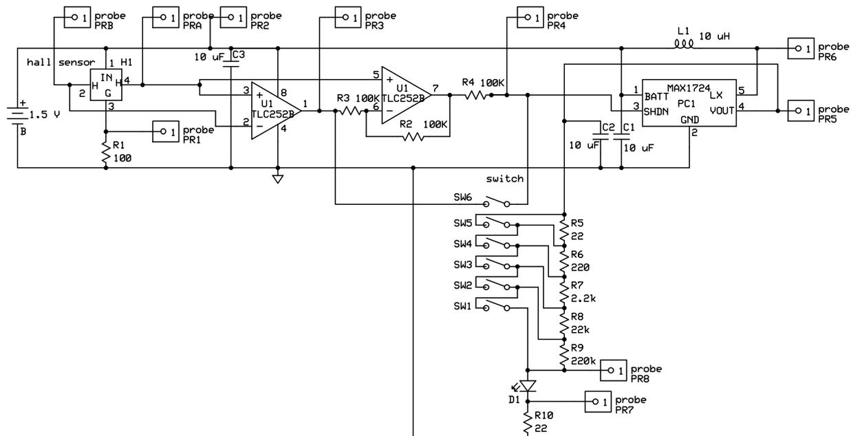
Test circuit for this lab. The top switch is labeled SW6 on the circuit board and the bottom one SW1. When a switch is in the ON position it is closed.
