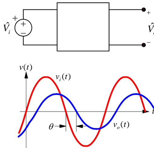
Figure 1. Input and output voltages of a two-port network.
