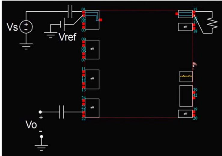
Fig. 10. Coupling arrangements for the input and output. IOCell3-5 are along the left edge.
