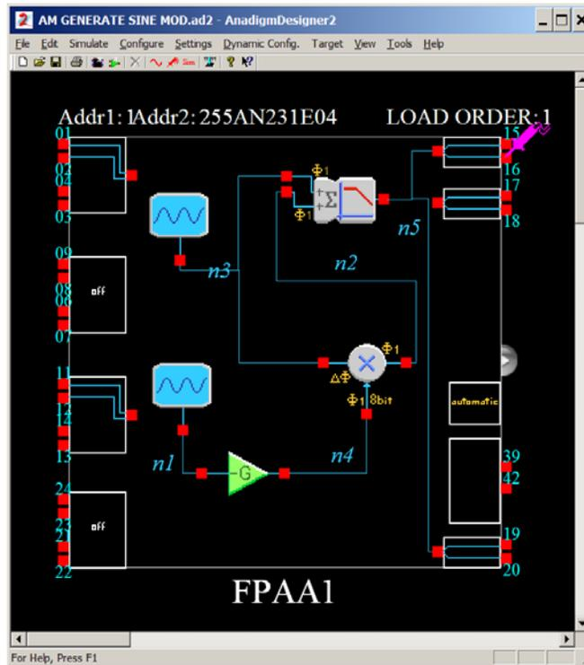
Figure 2. System for producing an amplitude-modulated signal.
