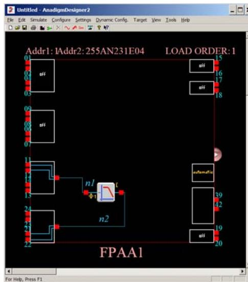
Figure 6. A filter module wired up to inputs and outputs.
