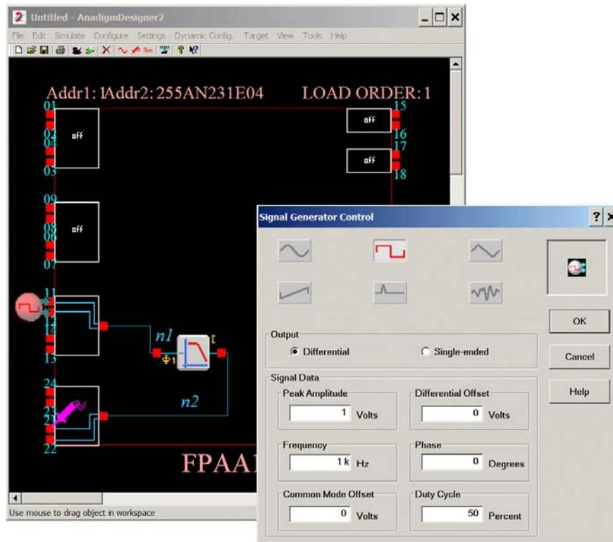
Figure 8. Configuring the signal generator for modeling the circuit performance.
