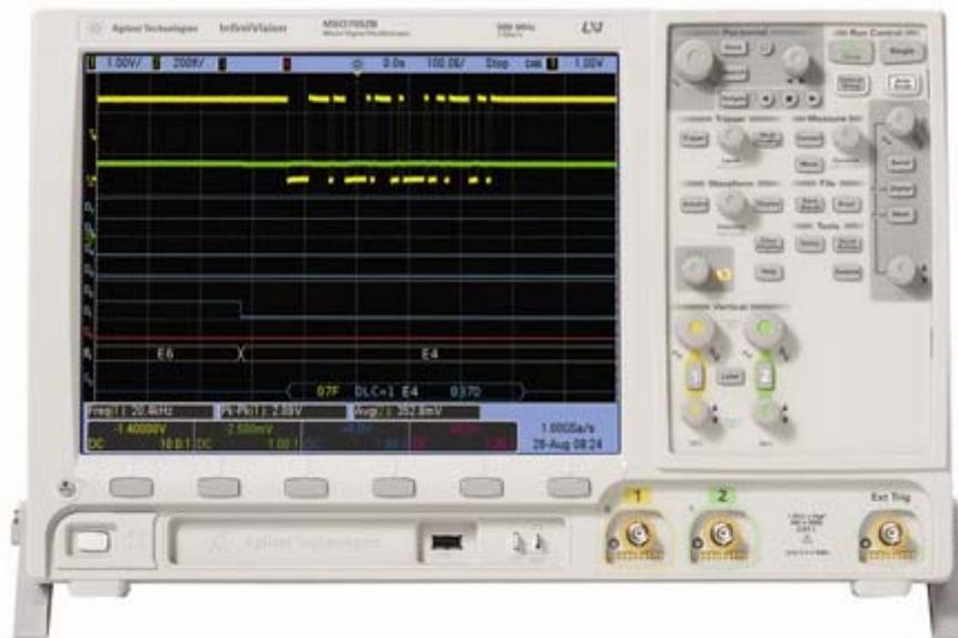
The user manual for the oscilloscope is located at <http://cp.literature.agilent.com/litweb/pdf/54695-97025.pdf>. See pg. 35 for an explanation of the front panel controls. Note that the AUTOSCALE button is often a good way to quickly set up a measurement. Not all measurements can be set up using the AUTOSCALE button, however, and it is necessary that you become familiar with other controls on the oscilloscope.
