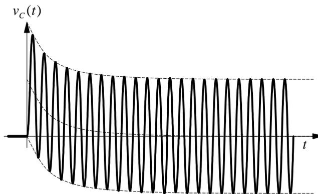
Fig. 4. RC circuit response to a gated sinusoid.
