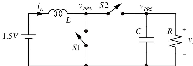
Figure 3. Simplified circuit diagram of the voltage converter circuit.
