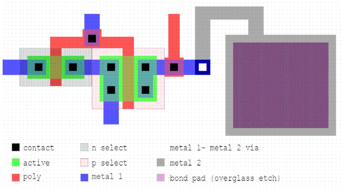
Figure 1. SOI-CMOS process and mask levels.
