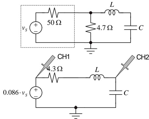
Fig. 4. Circuit for an  $RLC$  circuit with low  $R$ .
