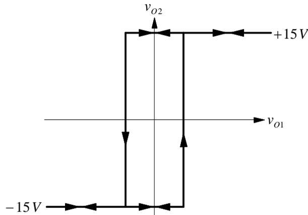
Figure 5. Transfer characteristic of Schmitt trigger in Fig. 4.
