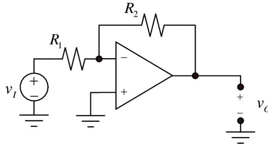
Figure 2. Inverting configuration.
