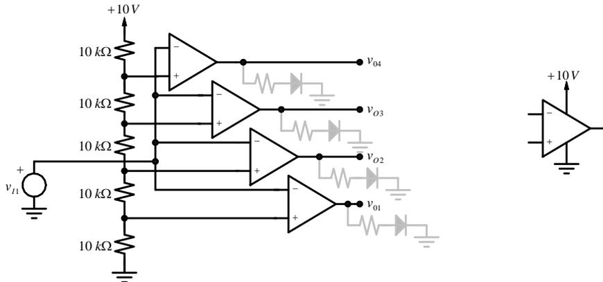
Figure 3. A flash A/D converter.
