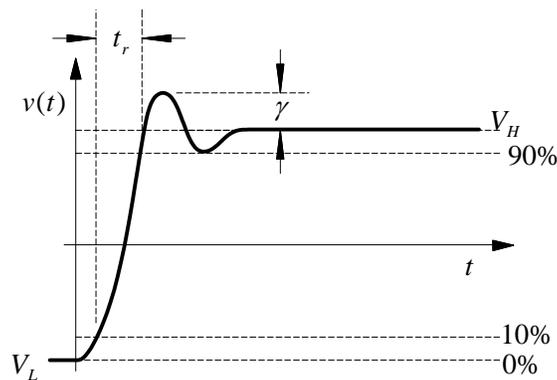
*Rise time* ( $t_r$ ) is the time it takes for the voltage to go from 10% to 90% of  $|V_H - V_L|$ .
