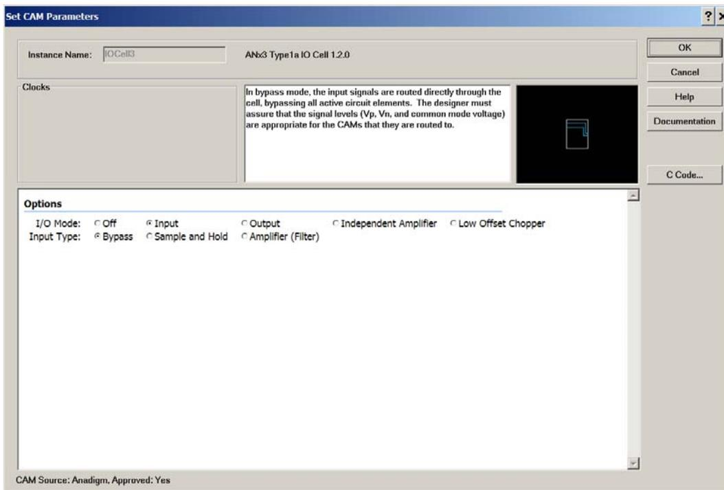
Figure 5. Configuration screen for inputs and outputs.
