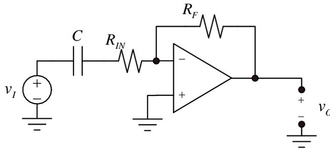
Figure 6. An active high-pass filter.
