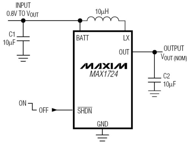
Figure 2. Connections to the MAX 1724 chip.
