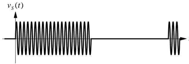
Fig. 3. Burst waveform.
