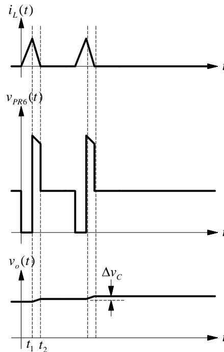
Figure 4. Waveforms in the voltage converter circuit.
