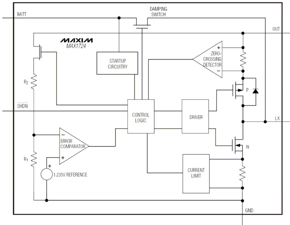
Figure 1. Block diagram of the MAX 1724 chip.
