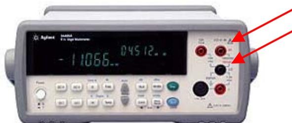
To set up for DC or AC measurements press the appropriate button in the top row. For measuring voltage or two-terminal resistance use the two right-hand upper terminals. The  $\wedge$  and  $\vee$  buttons set the range and  $<$  and  $>$  set the number of digits displayed.
