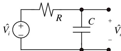
Figure 2. A passive low-pass filter.
