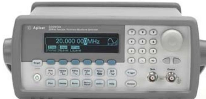
There are four standard waveforms accessible using the middle row of buttons. Each of these standard waveforms has several parameters which can be set (at minimum these include frequency and amplitude). The manual (found at <http://cp.literature.agilent.com/litweb/pdf/33220-90002.pdf>) contains a quick-start guide for this instrument.
