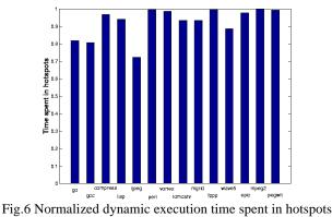
The amount of time a program spends in hotspots depends on the behavior of the program itself; Fig.6 illustrates this for the benchmarks that we tested. The average fraction of time spent inside detected hotspots is 92%, with the fraction being higher for MediaBench [27] than for Spec95 benchmarks [28].
