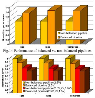
Fig.15 Energyxdelay product using multiple supply voltages
