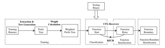
Figure 7: The BYTEWEIGHT function boundary inference approach.
