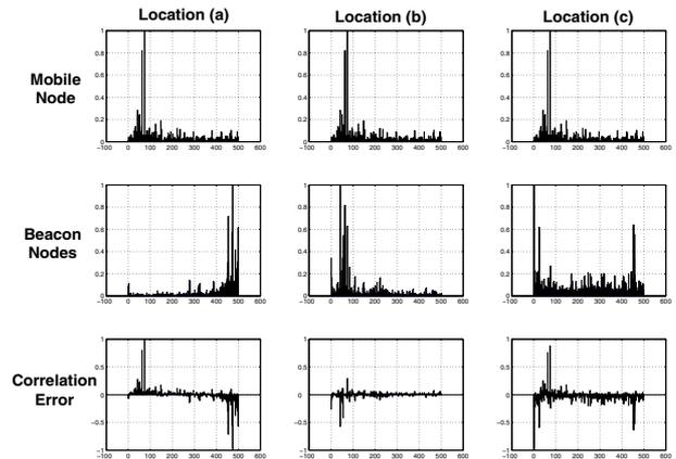
**Fig. 5. This figure shows a sample set of the spectral energy densities of 4 different time synchronized audio recordings. Each column shows the mobile node's data on the top as compared to the beacon at a particular physical location in the second row. The bottom row shows the difference between the top and middle signals. We present the signals seen by three beacons at three different locations. In this example, the mobile node was closest to location *b*, hence the least error.**
