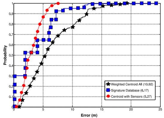
Fig. 7. Error vs Probability of 3 different localization schemes. Total cumulative error shown in parentheses ( $\times 10^4$ ).
