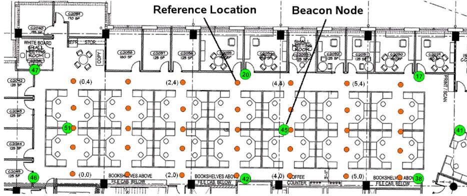
**Fig. 2.** Our experiments were conducted on the second floor the CIC building at Carnegie Mellon University. The 9 large circles with numbers inside them represent beacons, while the 35 smaller circles represent reference point locations.
