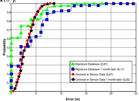
Fig. 8. Cumulative distribution error of the original signature database and then the original signature database against test points collected 1 month later. Total cumulative error shown in parentheses ( $\times 10^4$ ). The centroid weighting scheme with sensor data shows almost no change in performance over time.
