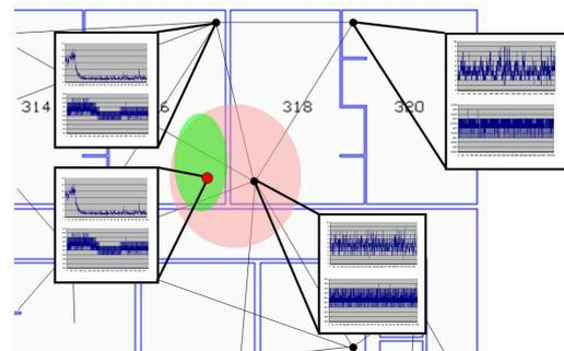
**Fig. 1. This diagram shows the floor plan of a nursing home outfitted with sensor nodes. The boxes associated with each node show sample sensor data. In this scenario, the micro-climate data helps associate the mobile node with the correct room instead of only basing the position on potentially misleading RSSI values.**
