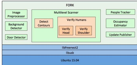
Fig. 4. FORK software architecture
