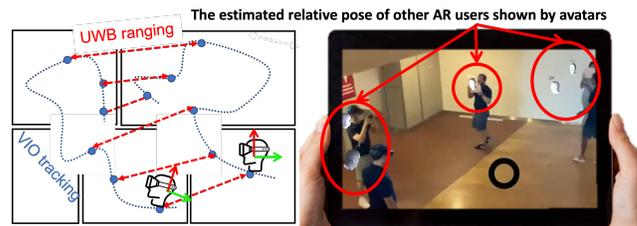
**Figure 1: Cappella offers a distributed infrastructure-free relative positioning framework that allows multiple mobile users to create a collaborative AR session even in non-line of sight.**
