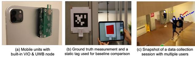
**Figure 5: System components, including UWB ranging nodes, ground-truth markers, and mobile tablet application**
