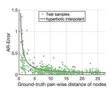
Figure 11: AR-specific error decreases over extended ranges due to lower sensitivity of AR displays
