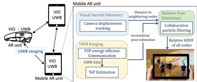
**Figure 2: System Overview.** A mobile user’s device locates several other target devices using a combination of VIO tracking and UWB ranging. 6DOF relative tracking enables AR overlays to be drawn on the display.
