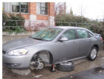
Figure 3. To test ECU behavior in a controlled environment, we immobilized the car on jack stands while mounting attacks.
