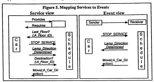
State—changing services and @T observer services map to events. Events are issued by a sender, received by one or more receivers, and may cause a state transition. (Conventional observer services are excluded from the definition of events (not given here) only to make the construction rules for state transition specifications easier to define. Such services, such as Last\_Floor? and Destination?, still, of course, constitute "object communication".)
