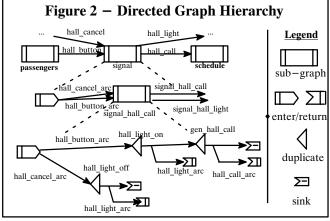
representational mechanism. Within a hierarchy of directed graphs, transactions flow among nodes which are "typed" in the sense that their operation is described by grouping them into various classes, such as those which duplicate transactions, those which delay them, etc. The
