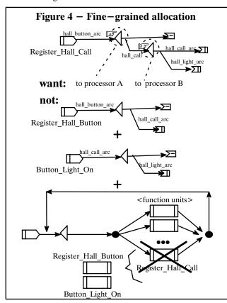
it is not possible to allocate the computational abstractions to separate processors unless they are made into separate sub-graphs. This can be done, of course, but at this point a figurative pencil which could group the abstrac-
