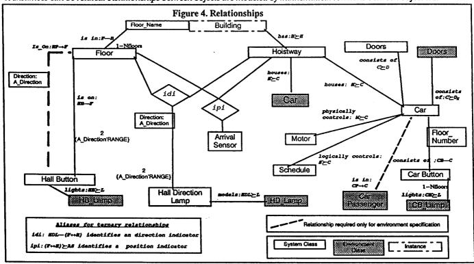
Arcs between classes represent relationships and are labeled, at minimum, with the relationship name and the "signature". (Some substitutes for the Z symbols are required and are listed in Table 1.) For example, Motor\_physically\_controls\_Car is a bijective function since the car uniquely determines the motor, and vice versa. Arcs may also be labeled with indicators for cardinality and for differentiating instances. For example, the ternary relationship idi, formally defined as:
