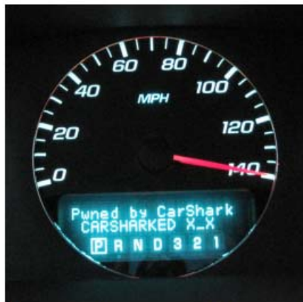
Figure 6. Displaying an arbitrary message and a false speedometer reading on the Driver Information Center. Note that the car is in Park.
