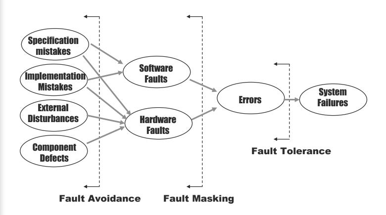
Barriers constructed by design techniques of fault avoidance, fault tolerance, and fault masking
