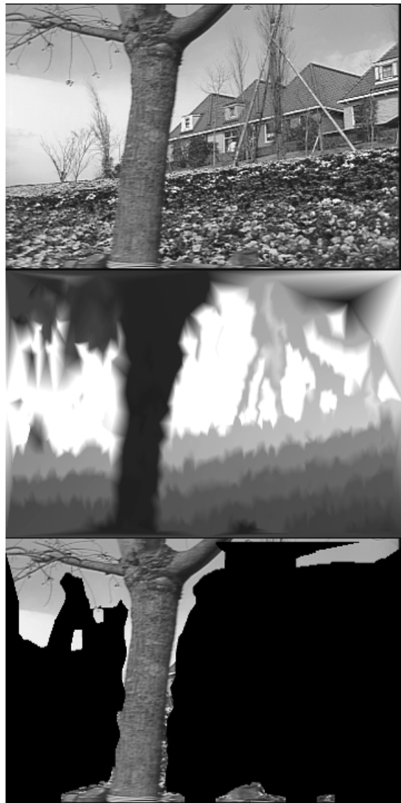
Fig. 15. An original frame of the “Flowergarden” sequence (top), the depthmap (middle) – light brightness means “high” depth, while low brightness means “low” depth, and the segmented (foreground) tree (bottom) using the results of the depthmap.
