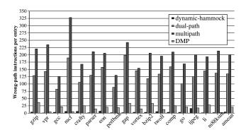
Figure 7. Fetched wrong-path instructions per entry into dynamic-predication/dual-path mode (i.e. per low-confidence branch)
