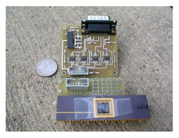
Figure 1. 2004 MEMS device and custom PC board with 4-channel amplification; housing (not shown) 45x50x90 mm
