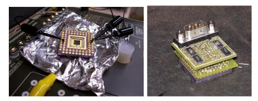
Figure 5. (a) 2006 MEMS device mounted in pin grid array package; (b) 2006 MEMS sensor system, with electronics, on steel plate.
